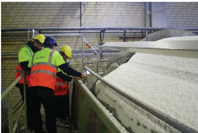
*The pulp is passed over a moving wire mesh, which helps to knit the fibres together and drain off the water.*
